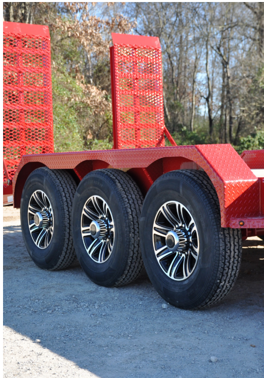
24,000 GVWR PACKAGE w/ ALUMINUM WHEELS & 3/16" SUPER HD FENDERS
