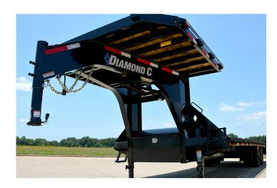
Place the deck on the neck of the trailer, ensuring the deck is centered on the neck. Make sure the back of the deck is flush with the rear neck uprights.
