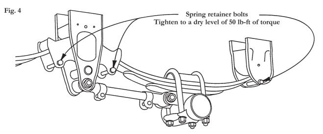
Loose fasteners that are allowed to operate for any period of time will result in irreversible suspension damage and possible loss of vehicle control. **Retightening a worn fastener will not correct a situation created by loose operation!**
