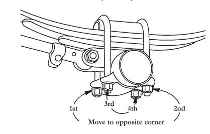
Always carefully inspect the spring and axle clamp components for any signs of wear or cracks, and replace if visible wear or cracks are present.
