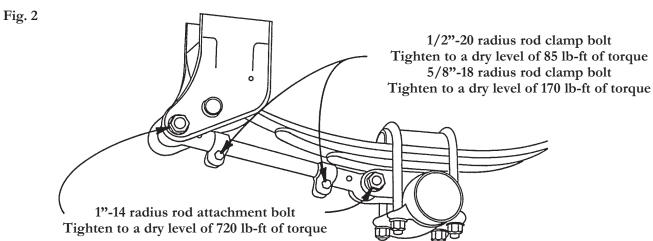
Loose operation of this bolt can result in wear requiring that new components be installed to avoid structural damage. During your visual inspection, if you observe any visible wear or loosening in the bushing, it is imperative that you immediately replace the radius rod bushing and bolt. Failure to replace these components will result in damage to the hanger, spring seat, and/or radius rod.
