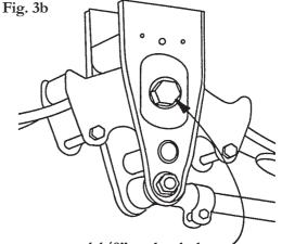
1 1/8" rocker bolt Tighten to a dry level of 790 lb-ft of torque
